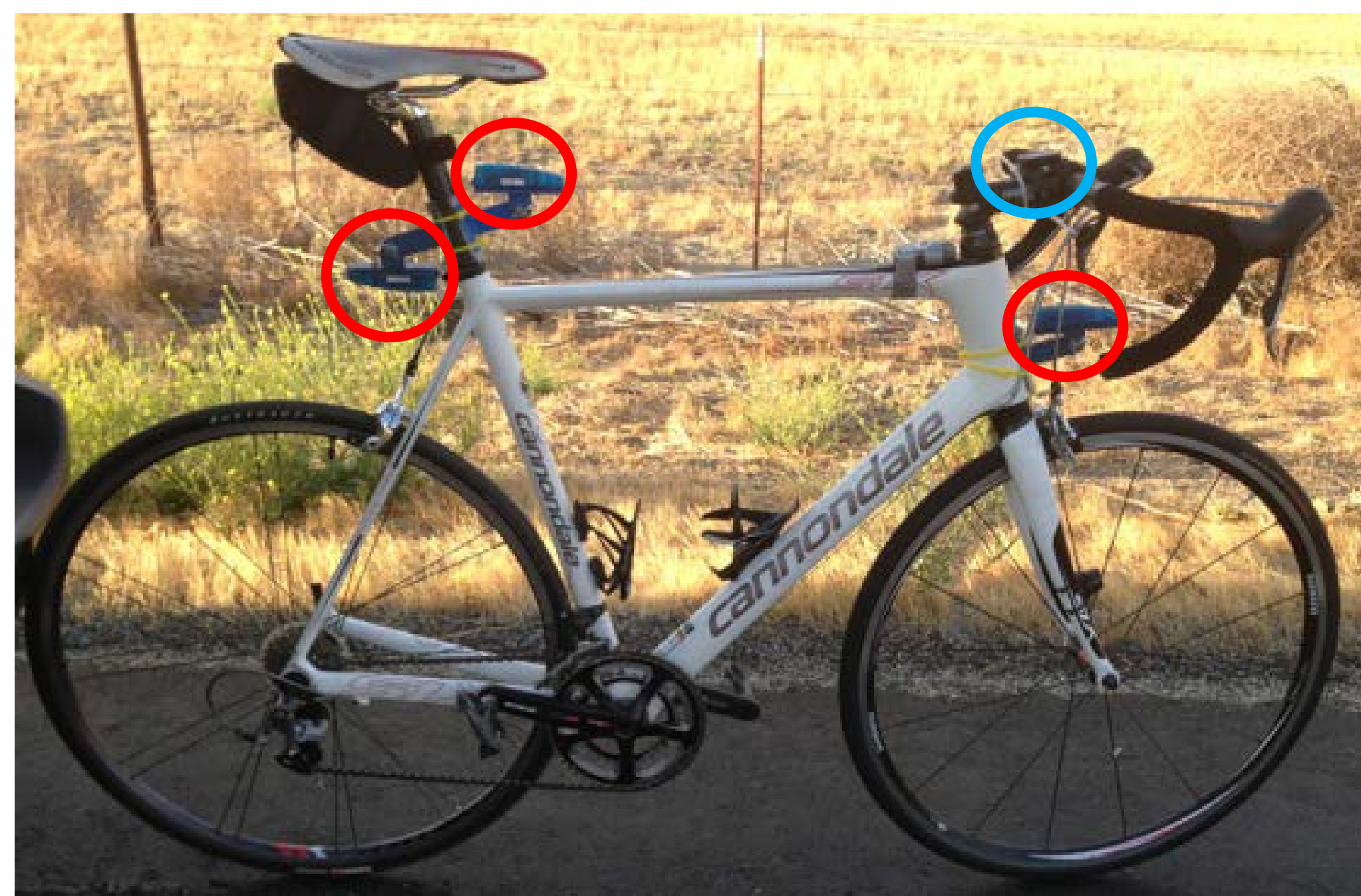
Bicycle instrumented with accelerometers (solid red circles) at three typical mounting locations and a GPS unit on the handle bar (blue circle).
